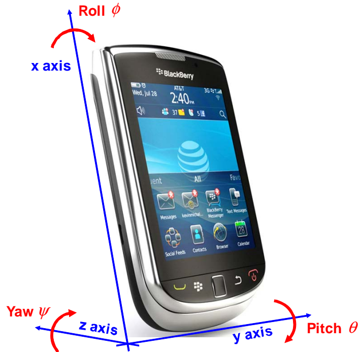
Figure 3. Definition of Coordinate System and Rotation Axes
