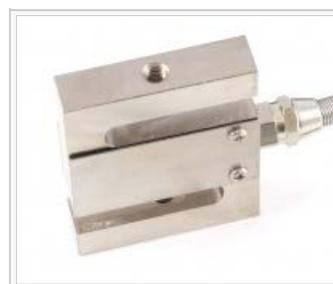
An S-type load cell. By pulling on both ends or pushing on both ends, the stress in the S changes and the cell's output changes.
