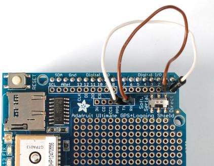
Finally upload the **Adafruit\_GPS->leo\_echo** sketch to the Leonardo, this will shuffle data from the GPS to the USB port
