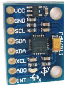
Photo: GY-521 breakout board
