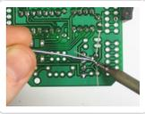
Turn the board over and solder/clip the three leads.
