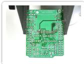
Get ready by placing the PCB in a vise.
