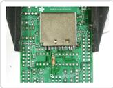
Form them into staples (as shown left with a 100 ohm resistor), then place them so they sit flat against the PCB, in the correct locations. Resistors don't have *polarity* so they can go in 'either way' and work fine!
