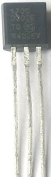
IC1 3.3V linear voltage regulator, 250mA current
