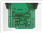
Next is **IC4**, the buffer to talk to the SD card. Match up the notch just like you did with the smaller chips.
