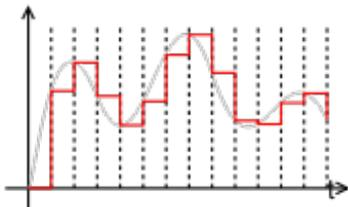
You'll notice it actually doesn't get the original waveform perfect. The more bits of digital data, the higher quality of audio reproduction. CDs have 16-bits per sample. While it would have been nice to have a 16-bit DAC, the best option for this design was a 12-bit dac. (That's still quite good.)
