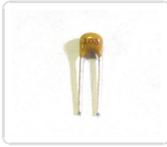
The way to tell the difference is look for the **103** printed on it. If it says **104** then it's a 0.1uF. Make sure it says **103**! This capacitor forms the output low-pass filter for the audio so its important to have the right value.
