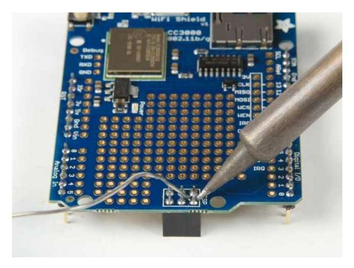
By default, SPI through the ICSP header is not connected. To enable the ICSP header connections, you'll have to connect three solder jumpers on the bottom of the CC3000 shield.
