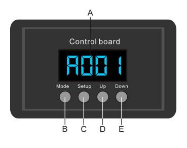
**A.** LED Display**B.** MODE Button**C.** SETUP Button
