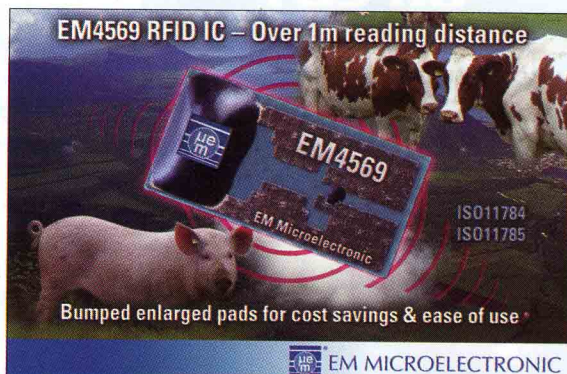
Figure 3. A typical 125 kHz tag used for animal tracking. Courtesy of EM Microelectronic.
